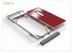
Once the 4 no.  $4.3 \times 40$ mm screws are in place, carefully open the door and lay it gently on the protected bearers.
