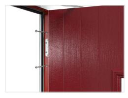
The pilot hole for the fixing should be countersunk to ensure the head of the fixing is slightly below the surface of the intumescent seal. Care should be taken not to over-tighten fixings. It is acceptable for the wall fixing to be positioned through the intumescent seal.
