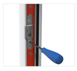
Checks should be made to ensure the lock hooks are engaging the keeps in a **central position** to ensure reliable operation of the lock throughout ongoing life service.
