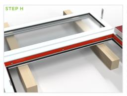
Drill 3 no.  $\times$  4.5mm diameter pilot holes through the head of the doorset frame and up into the toplight frame. Pilot holes should be located between 150mm and 200mm from corner of frame and at the mid point (just off centre) so you have 3 in total.
