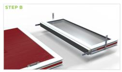
Screw (minimum size  $4.3 \times 40$ mm) fix  $1 \times VEKA$  steel frame strap to both vertical parts of the toplight frame. They should be positioned approximately centrally along the length.
