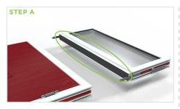
Inspect the coupler of the toplight that is factory fixed to the toplight frame. Confirm the grey intumescent 1mm thick pad that is applied to the coupler face where it will join to the doorset frame is not damaged. If it is damaged – do not proceed and contact Door-Stop for replacement.
