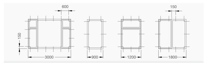
If fixing cleats is the chosen method of installation they should be attached to the outer frame starting at 150mm from the corner and thereafter at a maximum of 600mm centres. The cleats should be screwed into the mainframe in the central reinforcing chamber.
