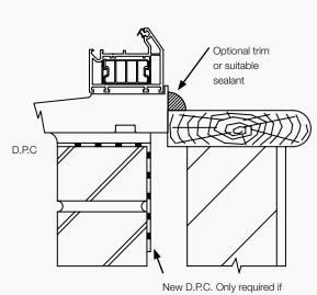
One was fitted originally And has been damaged in Removing the old window.
