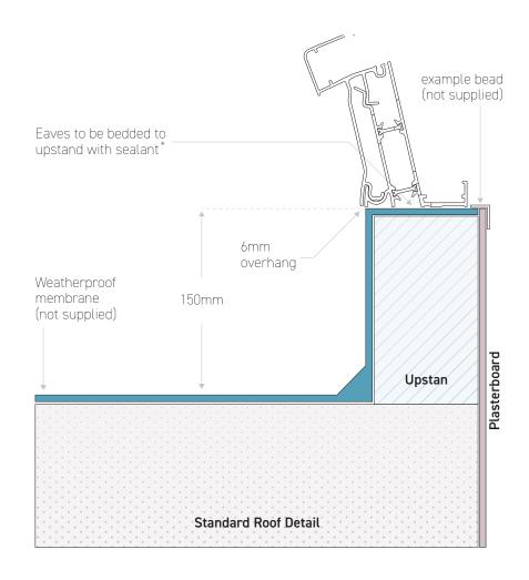
\*Sealant to be applied to the underside of the eaves as per installation guide instructions only
