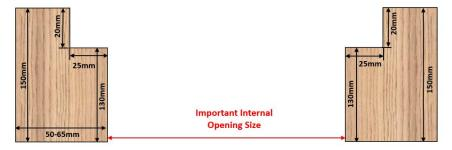
3. Apply weathering on top and down the side of the upstand (see diagram below)
