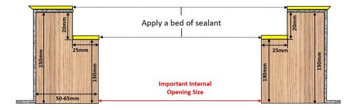
5. Secure rooflight on top of the beds of sealant.
